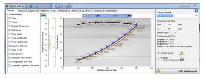
The comparative curves show that the propulsion efficiency is optimum for a rotation speed 160 revolutions per minute, the thrust of 105 newtons will be obtained at 300 revolutions per minutes and that to this rotation speed 300 revolutions per minute, la puissance a l'arbre sera de 200 watts pour un rendement de 0.8
